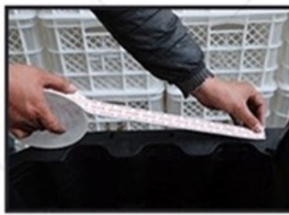
5. Foam sealant is stick to the edge of the bottom shell(No need to tear the upper layer)
